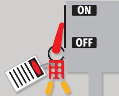
**Do not work on energized (hot) electrical circuits until all power is shut off and locked and tagged out (LOTO).**
