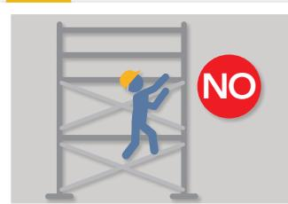
**Don't climb on cross braces or stand on guardrails.**
