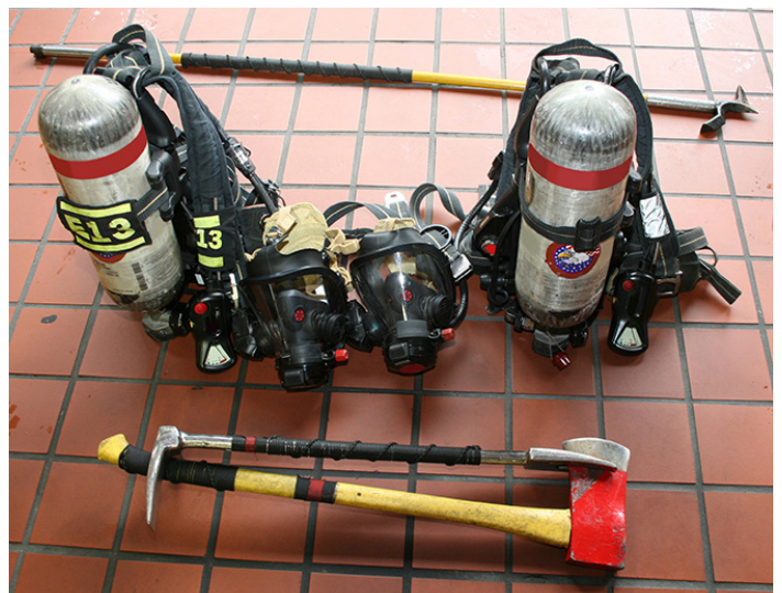
SCBAs and firefighting tools.
