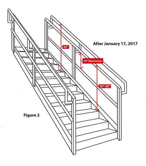
Figure 2. Depicts the heights of the handrail and the top rail of a stair rail system, when the handrail and top rail are separate; it does not show compliance with all provisions of the standard.
