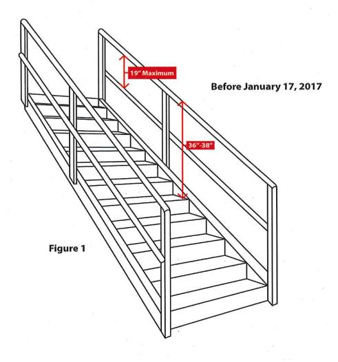
Figure 1. Depicts the height requirement when a handrail and top rail of a stair rail system are combined; it does not show compliance with all provisions of the standard.
