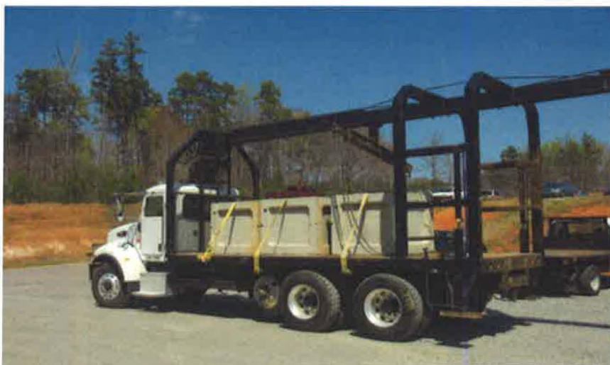
Photo 1: Septic Tank Delivery Rig
