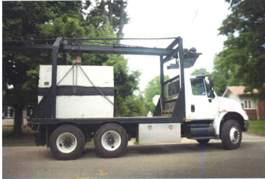
Photo 2: Septic Tank Delivery Rig
