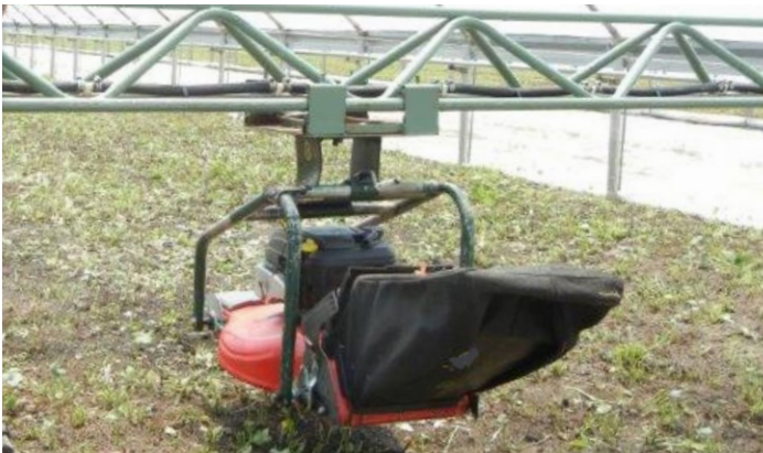
Modified mower mounted on boom.
