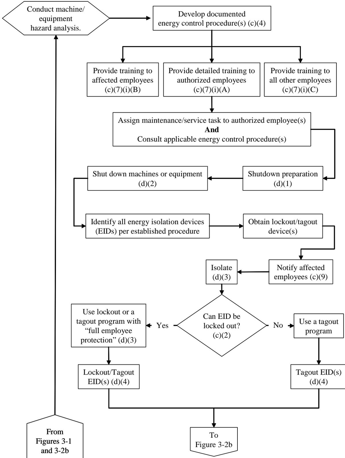
Figure 3-2b: Implementation of Lockout/Tagout (Part 2)
