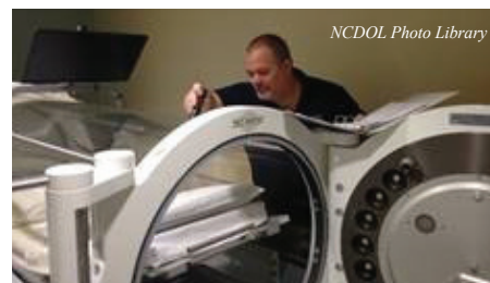
Boiler inspector John Kirkland uses a flashlight to check the serial number on one of the hyperbaric chambers at Wayne Memorial Hospital during a routine inspection. Hyperbaric chambers are inspected by the bureau every two years.
